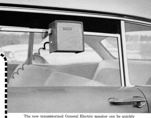
The new transistorized General Electric speaker can be quickly removed from its normal position on the firewall or dash and hooked over the top of either metal rimmed or plain window glass. The driver's range of hearing is greatly extended.
